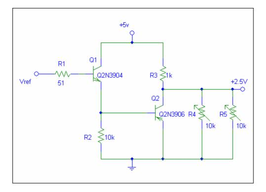
Figure 13. Voltage regulator circuit. [5]
