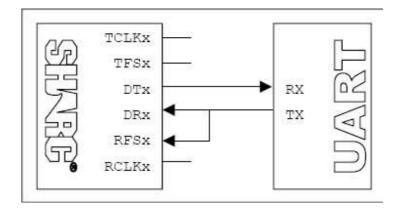
Figure 20. Physical connection between UART and DSP Serial Port [13]
