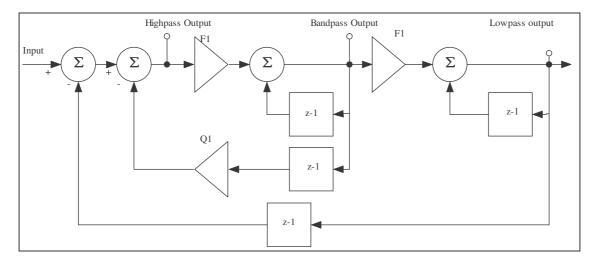
Figure 10. State variable digital filter, DAFX [2], chapter 2
