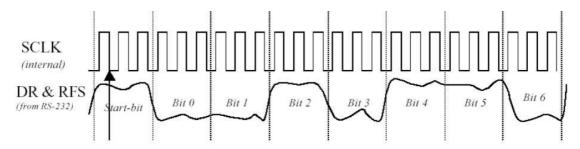
Figure 21. Over-sampling of incoming asynchronous data.
