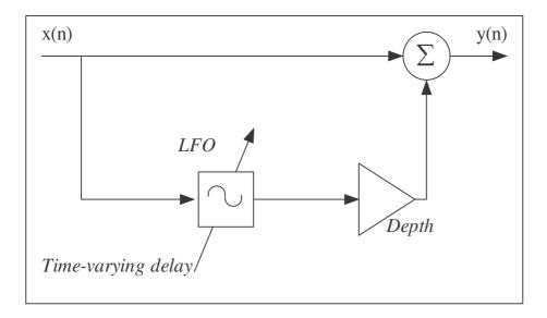
Figure 11. Flanger system block diagram
