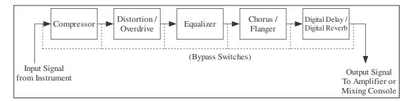
Figure 2. Typical Signal Chain for Multi-Effects Processors [1]
