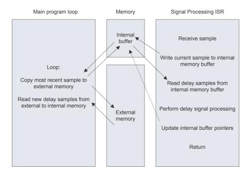
Figure 19. Block diagram of delay memory buffering application.
