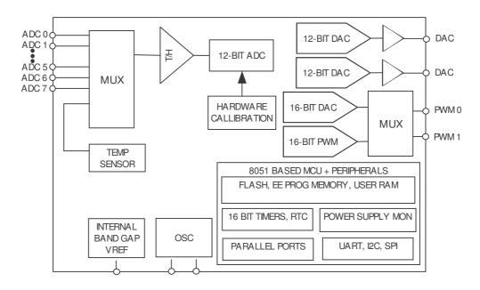
Figure 12. ADuC831 Functional Block Diagram [4]
