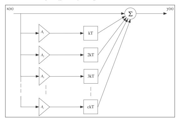
Figure 9 Block Diagram of Delay Effect
