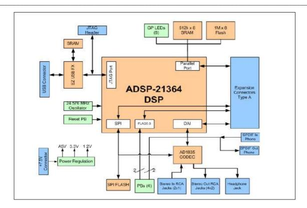
Figure 16. Block diagram of ADSP-21364 Architecture [9]
